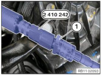
The compression adapter is used with the iMIB 100 bar pressure sensor (1) to test engine cylinder compression. For complete detailed information on this tool refer to ISTA Repair Manual section 11 00 039.
