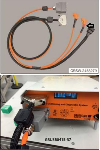
HV Battery Cell Module Charge Cable-
