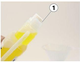
Pour the 60 ml of concentrate into the low temp coolant reservoir. **Do not spill** any of the concentrate.
