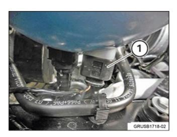
Replace the expansion tank and plug connection (1):
