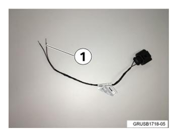
Cut back approximately 8 - 10 inches of the repair harness after the connector for coolant level switch. **NOTE:** The repair kit has enough wire to connect the coolant level sensor to the BDC. Only 8 - 10 inches of wire are needed for this repair.
