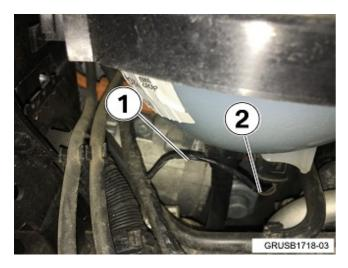
Once the expansion tank is removed, Remove the protective tape (1) approximately 4 inches away from the connector and cut the connector off the harness (2).
