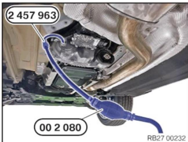
Extract the transmission oil from the transfer case (VTG) using special tool 0 493 337 (00 2 080) and special tool 2 457 963.
