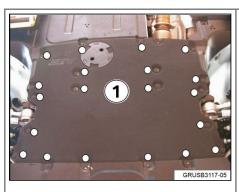
Remove the center lower protection cover (1). Tightening torque of screws when reinstalling is 3Nm.
