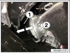
If there is no oil leak: Check for play in the output shaft (by hand) and pull the half shaft (1) as far as possible away from the extension housing (2).
