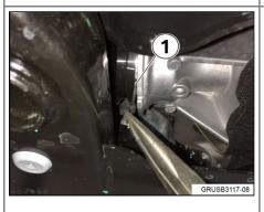
Insert a 3mm feeler gauge (3mm drill bit shown) into the gap between the output shaft and the extension housing (1). If the feeler gauge fits tight or will not fit (gap is  $\leq$  3mm) then no further repair is necessary. If the feeler gauge fits loose (gap >3mm), replace the output shaft. Follow Repair Instruction 31 60 000 Removing and installing/replacing left or right output shaft. (Right Side - KSD2: 31 60 504)
