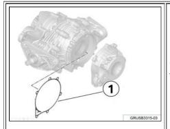
Gaskets are available through EPC (PN 33 10 7 601 264) for resealing the superimposing gear cases to the main differential housing (1)
