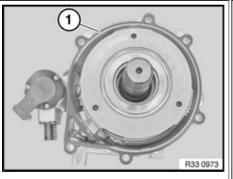
Both halves of the QMVH (1) will need to be resealed during the repair (do not repair only the side that is leaking).
