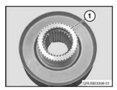
Apply lubricant P/N 83 23 0 443 864 on the input flange mating surface (1), as described in the illustration.
