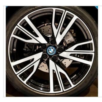
Vehicles delivered with wheel rim style 470 (shown) have directional wheels specifically for the left and right side of the vehicle.
