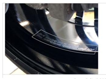
2. Raise the vehicle and locate the part number and batch number on the inside of the wheel rim.
