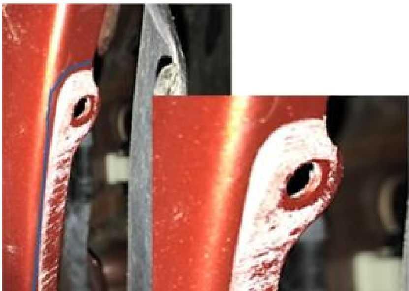
Damage version 3: Damage through the clear coat and paint down to the metal.
