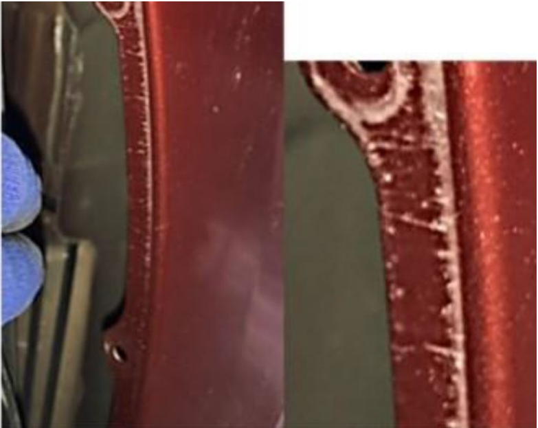
Damage version 2: Damage through the clear coat and paint. Damage must not extend all the way through to metal.
