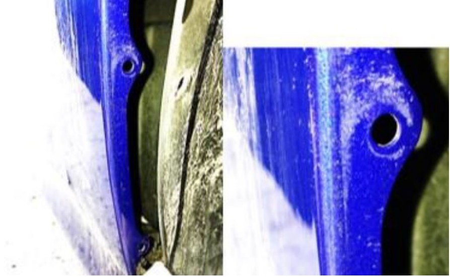
Damage version 2: Damage through the clear coat and paint. Damage must not extend all the way through to metal.
