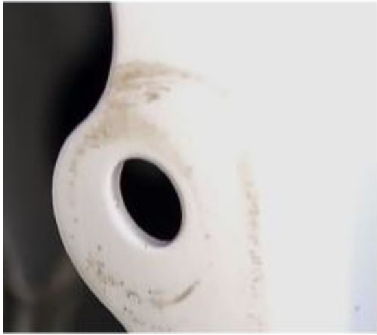
Damage version 2: Damage through the clear coat and paint. Damage must not extend all the way through to metal.
