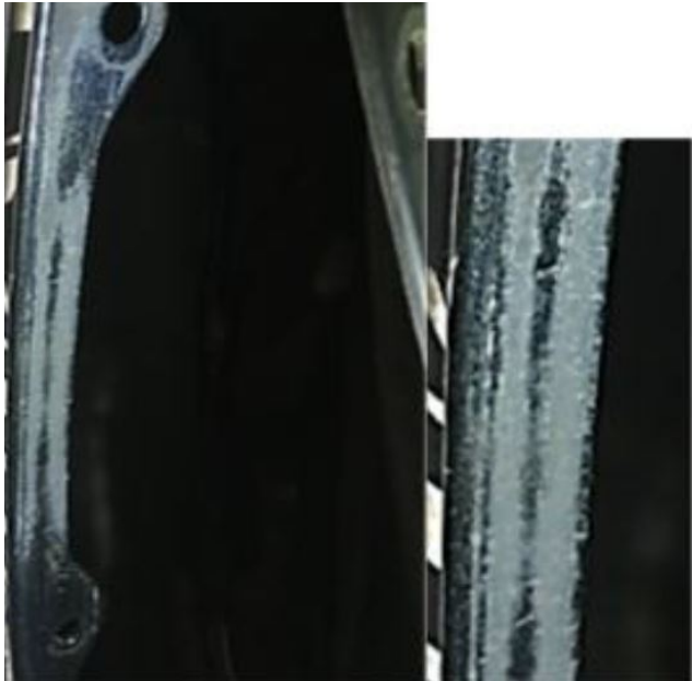
Damage version 2: Damage through the clear coat and paint. Damage must not extend all the way through to metal.
