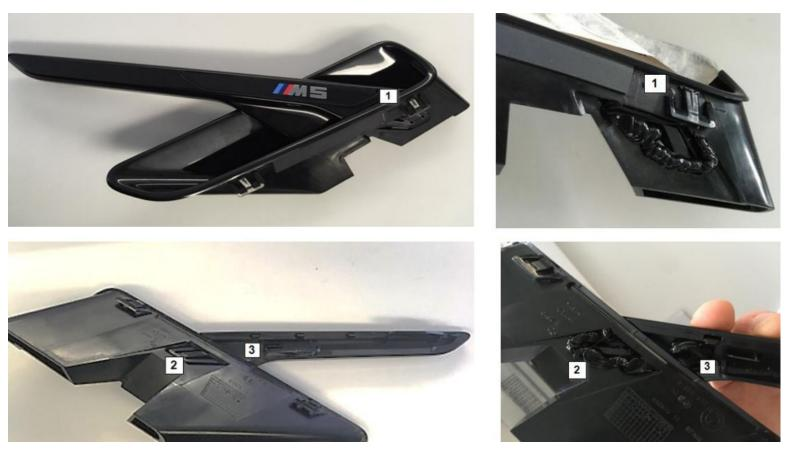
Note: The adhesive at position 3 will be used to bond the air duct cover to the fender. See step 4 for additional instructions for this position.
