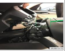
2. Disassemble the upper steering column shroud, following repair instructions REP 32 31 004 "Removing and installing/replacing steering column shroud upper section".
