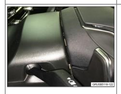
5. With the vehicle assembled, visually inspect the gaps again to verify that they are uniform as seen in the photo to the left. Verify that no noise if present after repairs.
