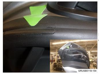
If the weather strip has visible separation at the glued area as shown to the left, it will require replacement.
