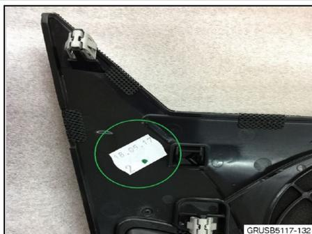
2. Make sure the replacement part has a "green dot" on production code label (as shown on left). The production date should be 18.05.17 (DD.MM.YY).
