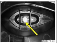
**Before** installing the reinforcement element, make sure the bushing has been removed as shown in the picture.
