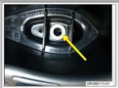
Remove the bushing from the left side support element as shown and discard. The bushing is no longer required.
