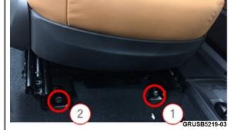
Note: Replace the bolts (Collar bolt M10 X 28).
