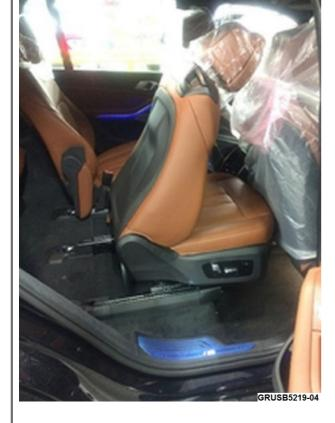
Move the seat fully forwards and keep the seat at its highest position (up and front) to gain access to the rear bolts.
