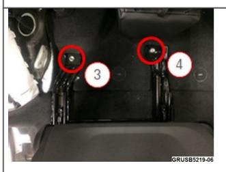
Remove bolts 3 and 4 with the Wheel Lock Removal kit, special tool 0 495 223 (36 1 325), Socket # 32.
