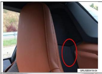
1. Completely open the convertible top to gain access to the main convertible top hinges (circled) on both sides of the vehicle.
