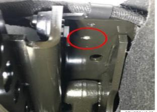
2. Inspect both hinges for signs of interference between the adjustment stop screws and convertible top hinges.
