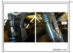
2. Using a cable tie (part number 31 13 1 357 599), attach the tube to the holder observing the dimensions shown.
