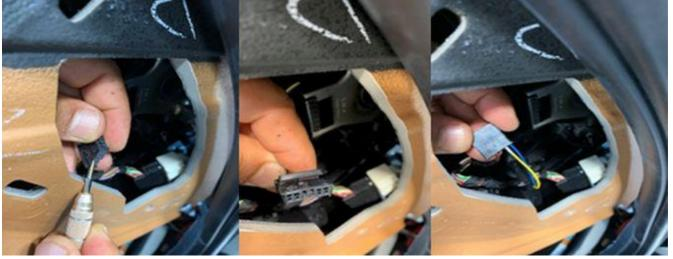
Route and fasten the wiring harness such that no chafe marks can develop as seen below. Wrap in adhesive tape and secure any extra wire length.
