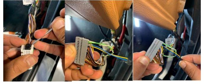
3. Open the connector X673\*1B with tool 94018 or 89090.
