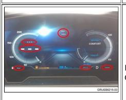
Incorrectly functioning Instrument Cluster with numeric displays displaying only dashes
