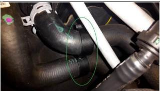
Close up view of spacer installed.
