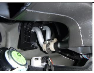
Tape the two heat exchanger lines with a felt strip (part number: 51 45 2 353 024) 4-5 inches (10-12 cm) long around each of the lines. Secure the lines together using a worm-type hose clamp (part number 07 12 9 952 117).
