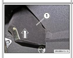
Correctly position the air freshener cover (1) and press firmly in the direction of the arrow until the latches engage.
