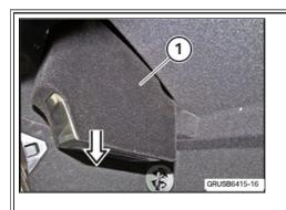
Open the lid for the glove box. Remove the cover (1) in the downward direction of the arrow
