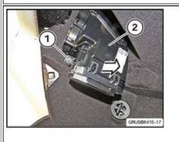
Loosen screw (1) and remove the air freshener (2) with forceful pull in the direction of the arrow.
