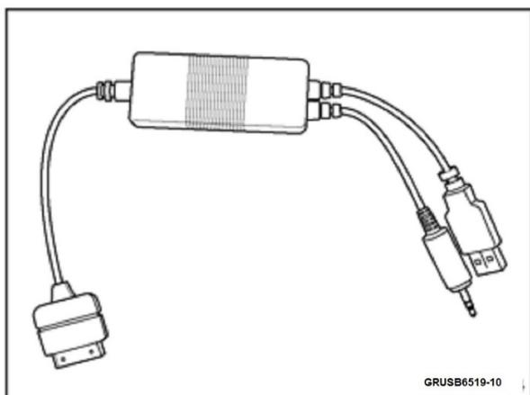
Apple iPod devices must be connected to the vehicle through the adapter cable provided (Y cable from 30-pin-connector to USB and AUX-In).
