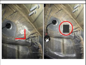
Remove the emergency horn with tilt sensor located by the wheel arch liner.
