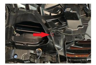
5. Repair all damaged wiring. Wrap wiring in abrasion resistant tape. See example photo of possible damage location.
