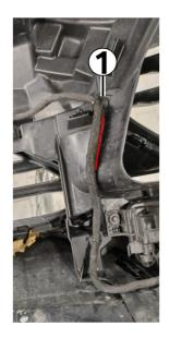
6. Install wiring harness into 70 mm length of corrugated tubing.
