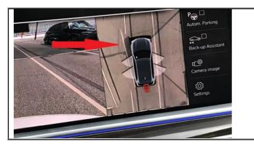
The arrow identifies the line which is shown as not parallel or straight alongside the vehicle.
