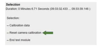
When the test plan job selections are displayed as seen in this image, select the job labeled "Reset camera calibration".
