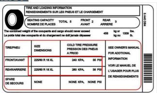
During vehicle production, a tire pressure label containing the incorrect tire size was installed on the vehicle's driver side "B" pillar.
