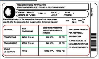
Replace the tire pressure label with one showing the correct tire size for the vehicle equipment.
