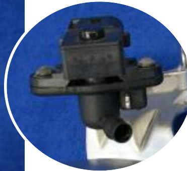
Secondary Air Valve and Pressure Sensor
