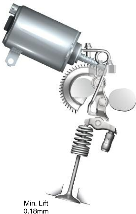
Valvetronic II at minimum valve lift
