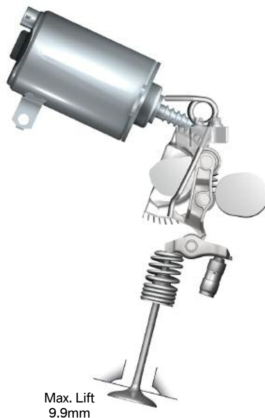
Valvetronic II at maximum valve lift
