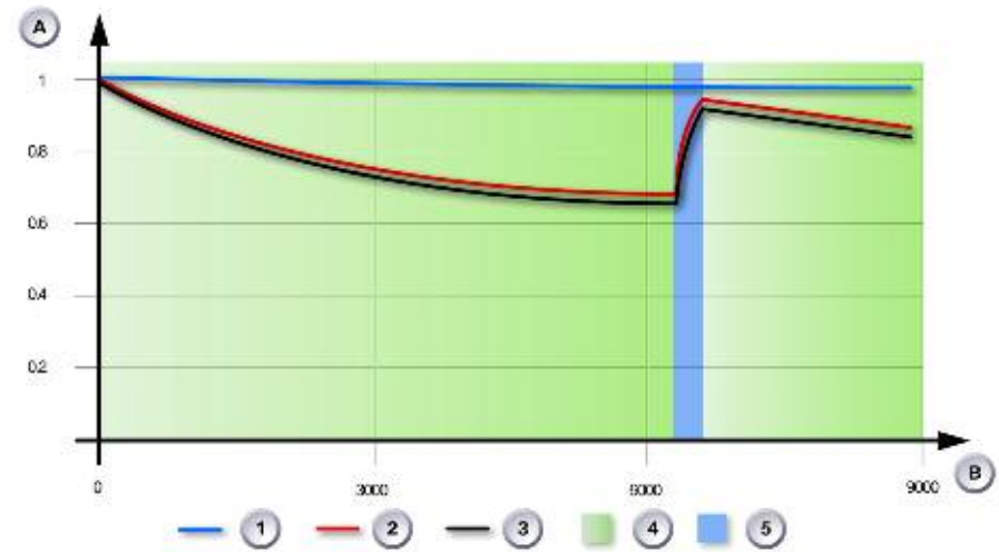
Storage capacity reduction of NO x storage catalytic converter with regard to sulfur.
