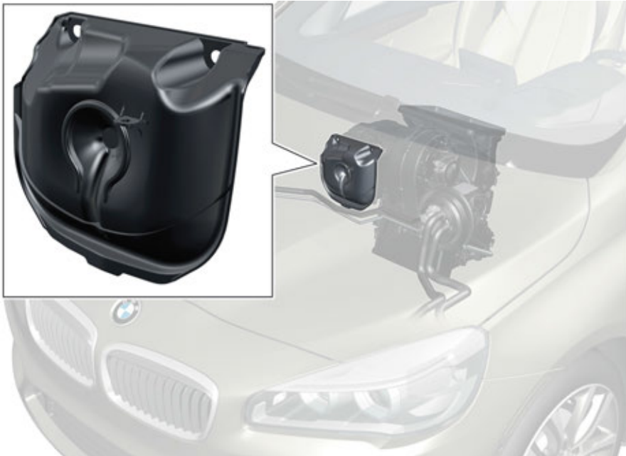
F48 air/water separation (Venturi adapter)
