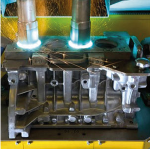
Electric arc wire spraying method, Bx8 engine
