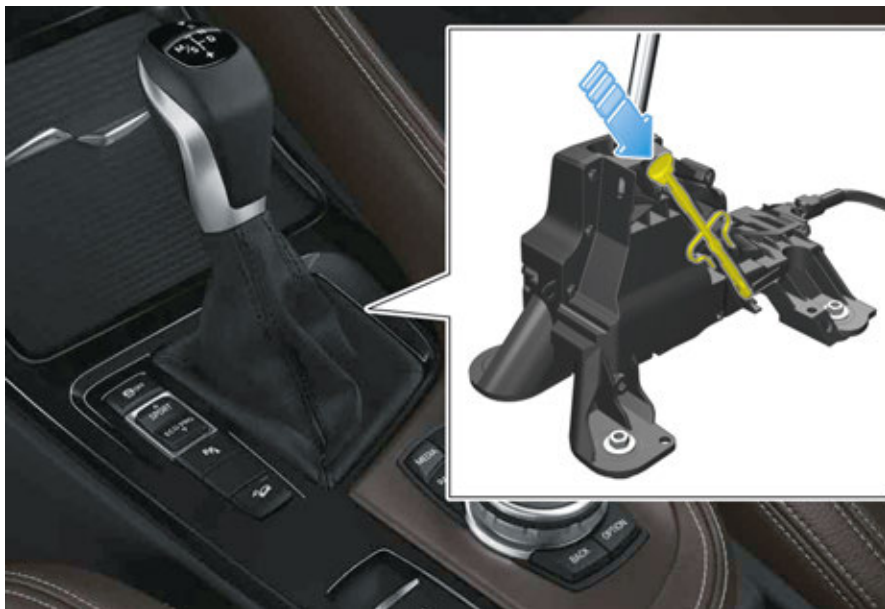
F48 Manually unlocking the drive position lock
