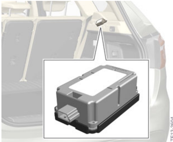
F48 Installation location of the remote control receiver
