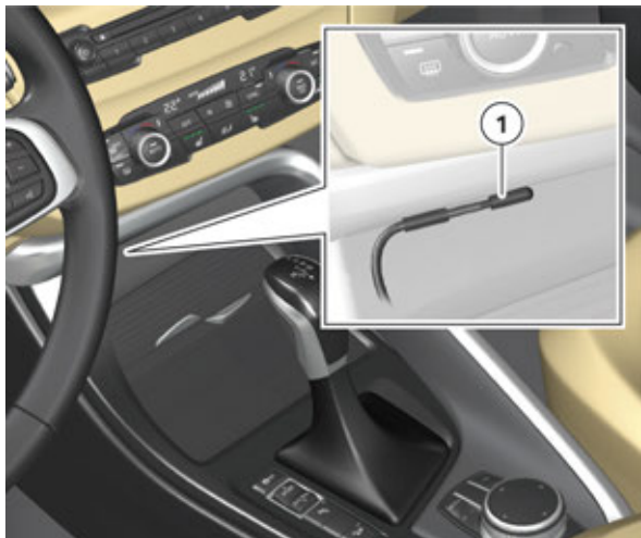
F48 installation location of Bluetooth antenna
