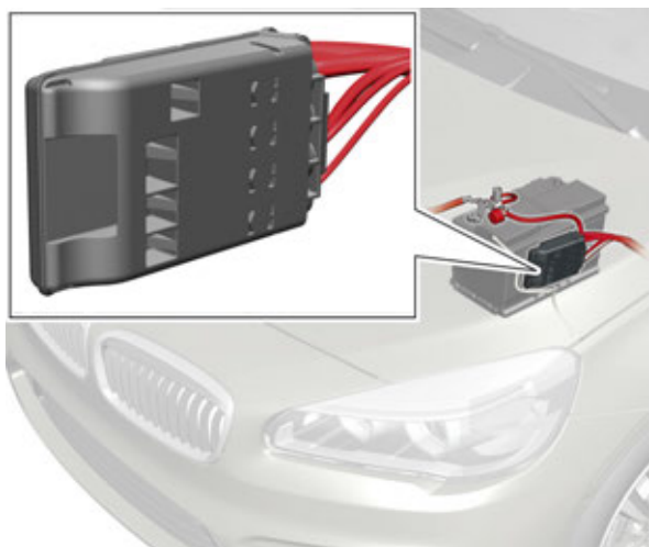
F48 Battery power distribution box
