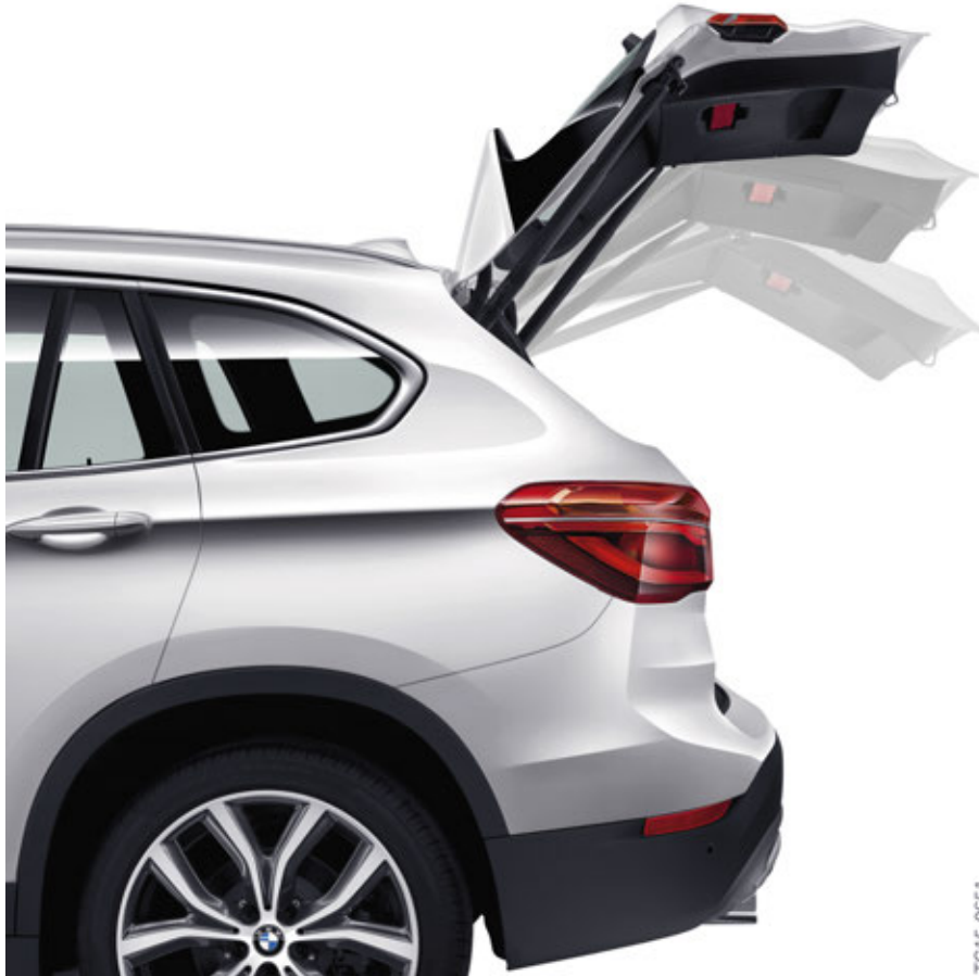
F48 Automatic operation of tailgate
