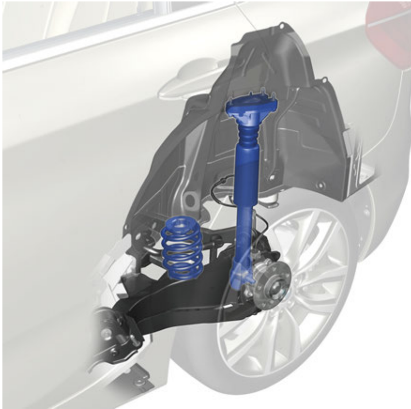
F48 suspension/damping action, rear
