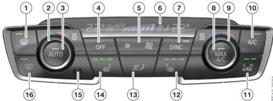
F48 IHKA control panel
