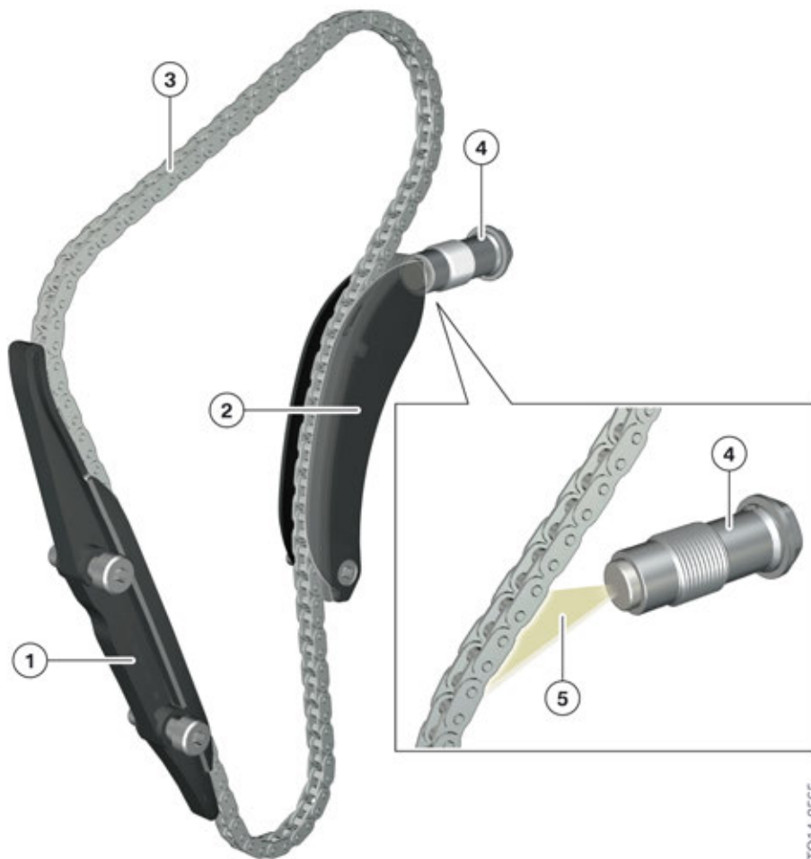
Lubrication of top chain drive, B46 engine
