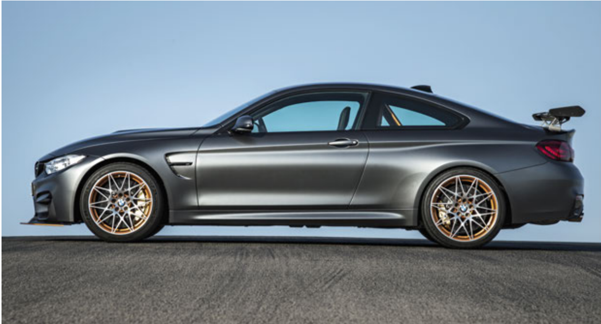
F82 GTS, side view, rear spoiler winglets mounted for Euro specification
