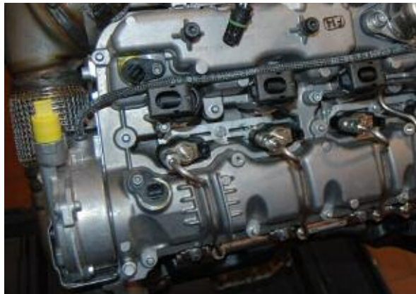
N63 Vacuum pump location
