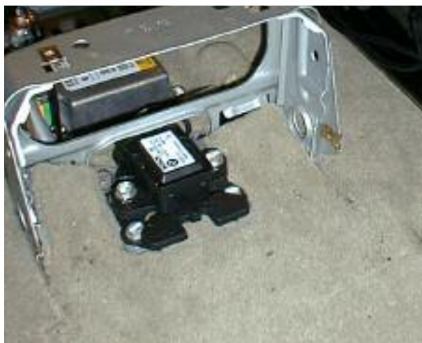
Location of the Rotation Rate/Transverse Acceleration Sensor under the center console
